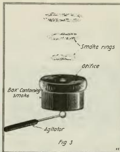
The Vortex Ring Smoke "Gun." Every Time the Bottom or Diafram of the Box is Struck, a Smoke Ring Issues from the Small Opening in the Top of the Box.
